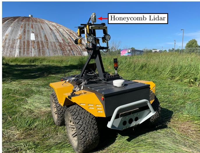
Figure 4.5: This picture shows our Clearpath Grizzly UGV used for data collection, equipped with a Waymo Laser Bear Honeycomb lidar.
