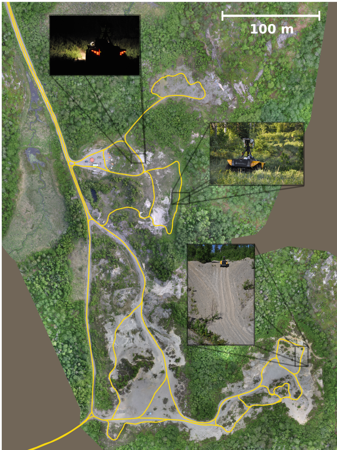
Figure 2.1: An orthomosaic map of the 5 km network of paths at the Ethier Sand and Gravel in Sudbury, Ontario, Canada, constructed during VT&R2 field testing. Image credit: Paton et al. [1]
