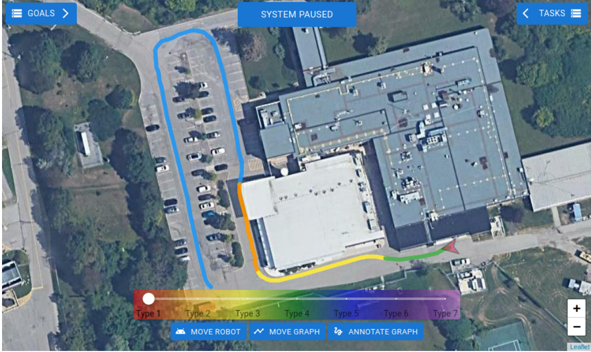
Figure 4.3: This figure shows the updated VT&R3 GUI for specifying and visualizing the safe corridor information. The slider at the bottom is used to specify the safe corridor width during each teach pass, and the paths are colored accordingly.
